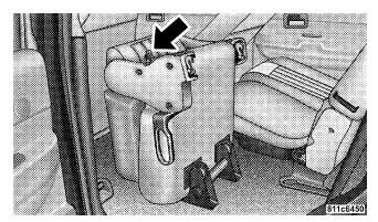
**NOTE:** The secondary lever on the rear of each cushion allows third row-seat passengers to release the latches and fold the seatbacks when exiting the vehicle.
